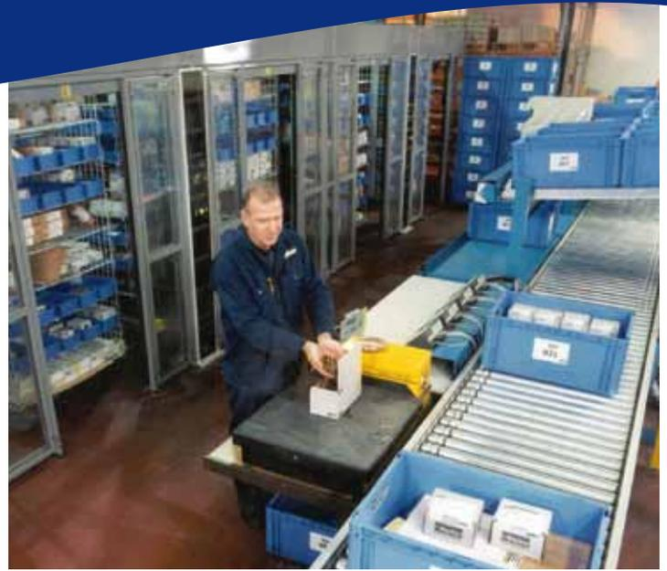
Diamond Phoenix FasTree™ pick-to-light technologies are utilised to ensure order accuracy and integrity.
